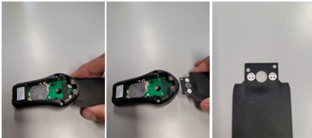
3. Put the cover back on and turn the ring 90° clockwise.
