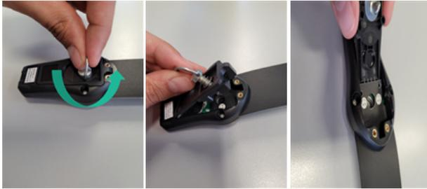
2. Take out the strip, insert a new strip, and make sure to align the connectors on the strip and the printed circuit correctly. There are emoticon indicators on the strip. The strip is inserted correctly when the smiley faces are facing up.
